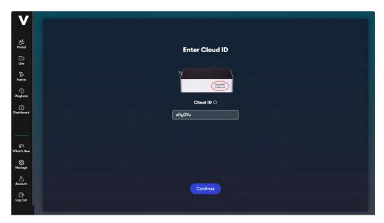
• When the Cloud Adapter is discovered, it will be linked with the account. Click 'Continue'. Videoloft will then discover all cameras and recorders connected to the same network as the Cloud Adapter.
